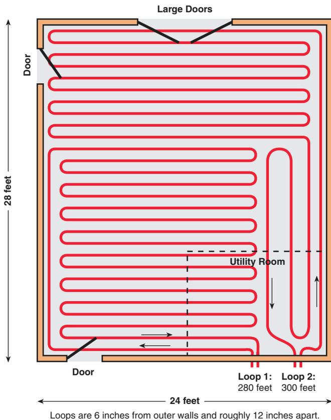
I felt that 2 inches would be too thin, and the concrete contractor refused to pour less than 3 inches due to the risk of damaging or exposing the tubing. The 3 inches still allows me to use a single household thermostat to control the heating, though it is less responsive. I'm still testing, but I believe that the system can raise the building temperature by about 3°F (1.6°C) per hour.
