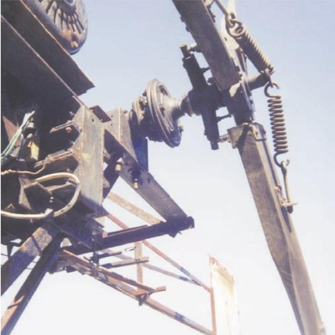
**Detail of the underside of the drive shaft mounting.
