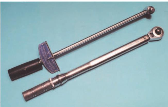
You might not feel like putting a torque wrench on every fastener you put on your conversion. Few people do. However, as a minimum, you must torque any fastener that is helping to support a lot of weight or is part of a rotating mechanism. These are the areas where failure is likely and will cause the most damage.
