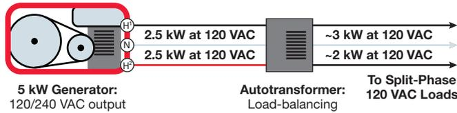
Current-limit settings on an inverter-charger allow maximum use of generator output without overloading.
